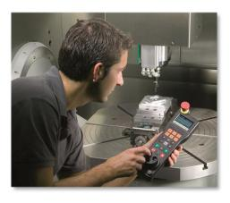
The transmission range is amply dimensioned. If you should nevertheless happen to come near the edge of the transmission area, which is possible with very large machines, the HR 550FS warns you in time with a noticeable vibration alarm.
