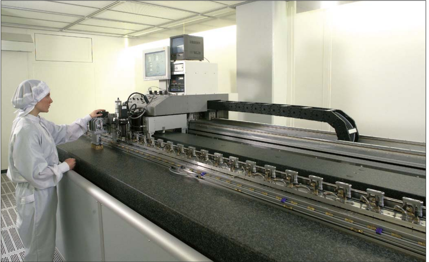
Figure 9: For each scale of an exposed linear encoder, HEIDENHAIN uses a special measuring machine to ascertain the baseline error in a defined interval.
